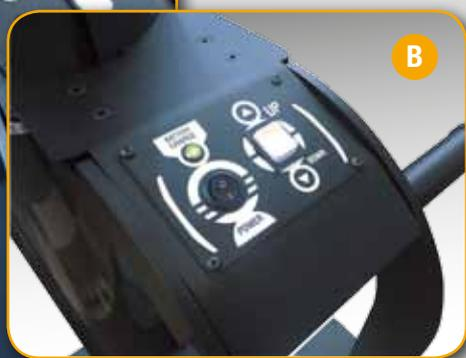
**EN** → • **Automatic and precise:** thanks to the UP & DOWN selector the wheel can be lifted and its mounting/demounting position can be accurately centred.
