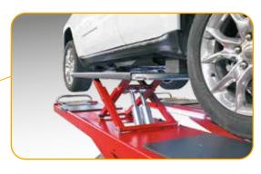
•Lift table with double lifting cylinder to ensure a constant parallel lift movement.
